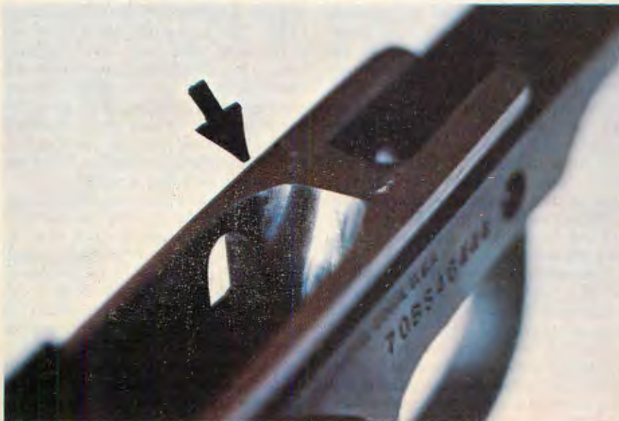
Below: Critically necessary part of Combat conversion of .45 auto is "throating" of weapon to insure maximum feeding reliability with all types of ammunition and bullet shapes. Most standard autos will feed reliably only with ball or round-nose lead ammunition.
